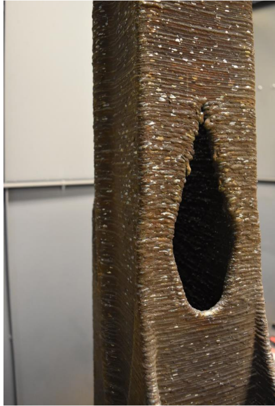
Figure 41. Cut-out hole in printed arm.
