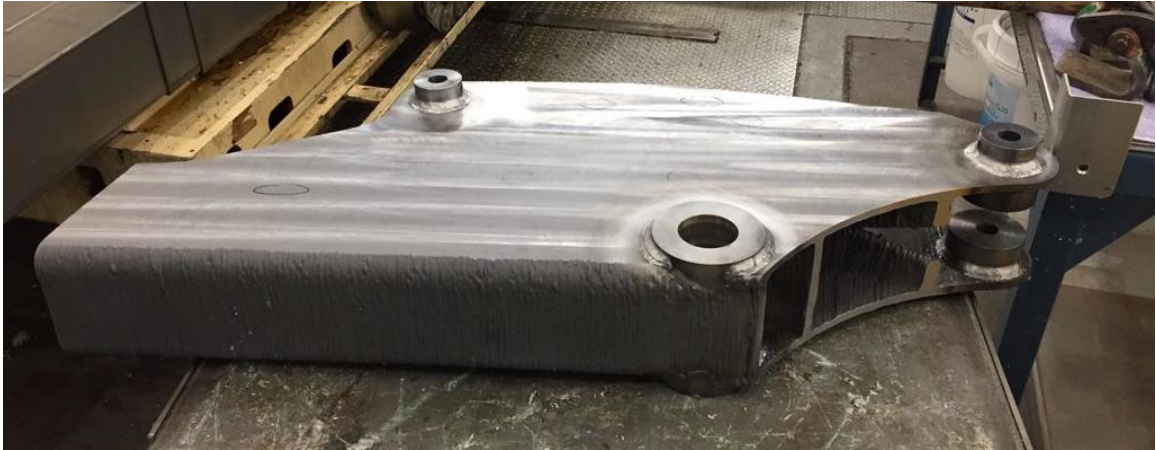
Figure 44. Alternative view of the machined arm and the welded-in sleeves.
