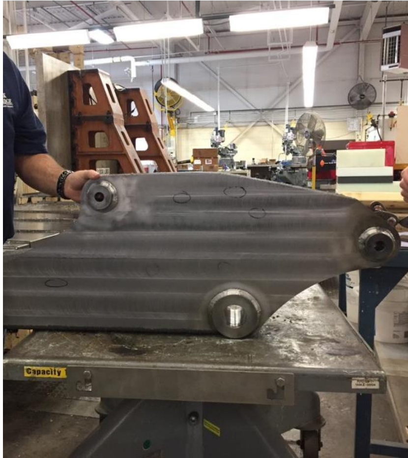
Figure 43. Test section of the arm to demonstrate finished surfacing and welding of the bearing sleeves.
